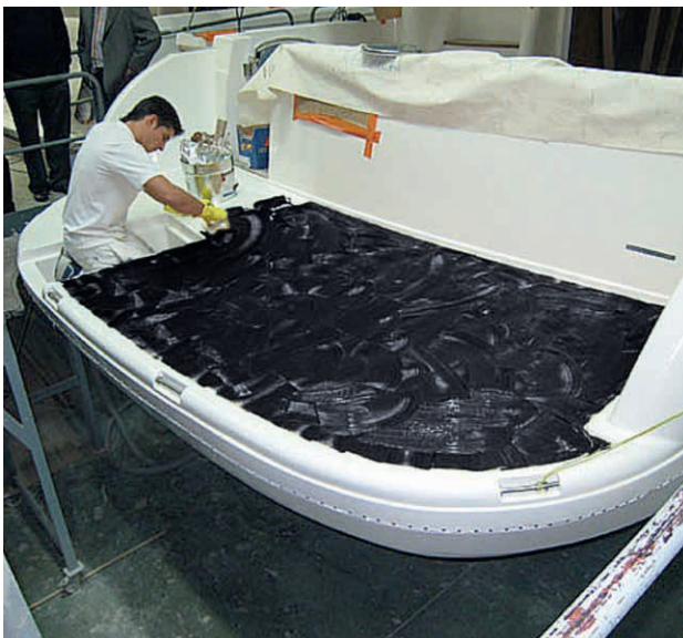
Fig. 26 Application of Sikaflex®-298
