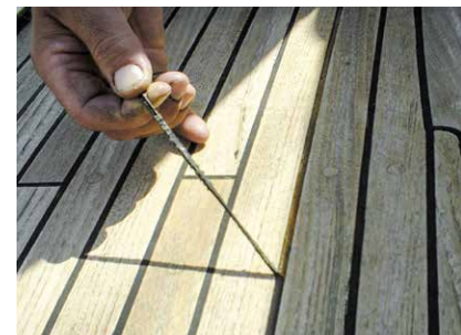
Fig. 45 A triangular cut of the old caulking being removed manually
