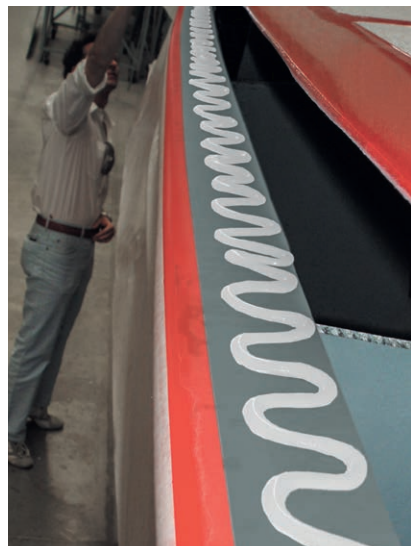
Fig. 9 Hull and deck are brought together
