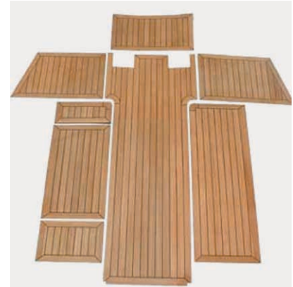
Fig. 22 A prefabricated teak deck is laid out in preparation for fitting
