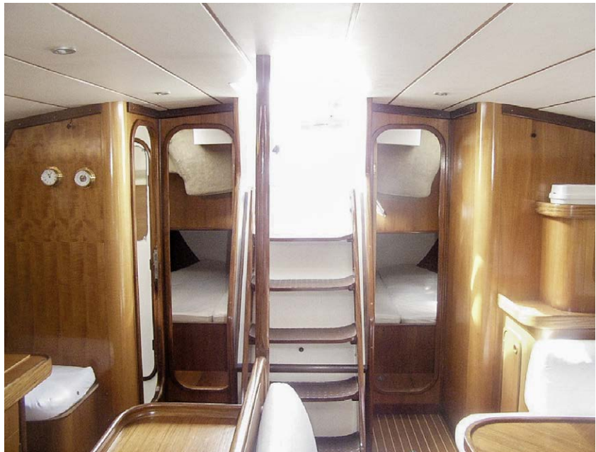
Fig. 13 High-quality lightweight panels finished in traditional high-gloss wood veneer and bonded using Sikaflex®-292i
